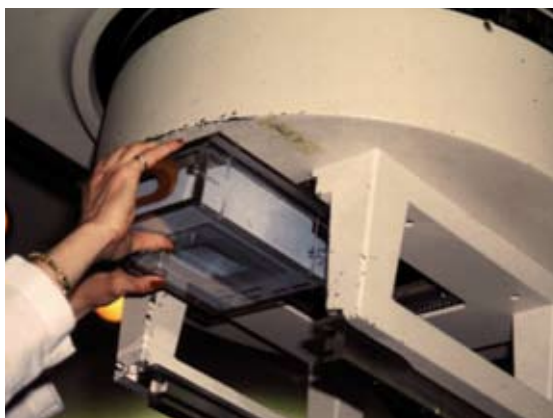
Figure 5: Demonstration of IMRT Compensator Box Insertion. Block Tray is Another Location for IMRT Compensators
